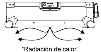
As you can see in the upper picture, the heat radiation is envoy to outside of flight case to prevent engine failure..
